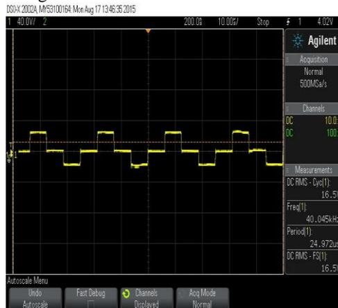
Fig. 22. Voltage across switch S1a
