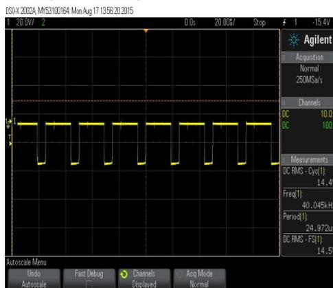
Fig. 26. Voltage across diode 1
