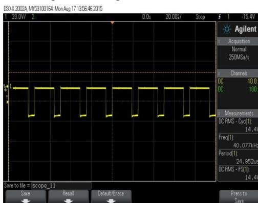
Fig. 27. Voltage across diode 2
