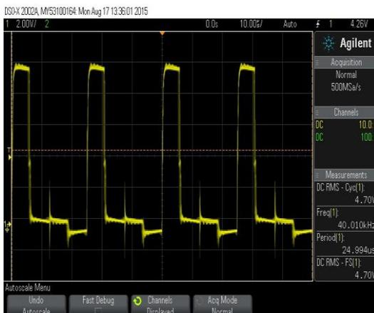
Fig. 20. Pulses for switches S1a and S1b
